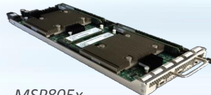
MSP805x Intel CPU+GPU E3-1578Lv5 HD & 4K Media Transcoding
